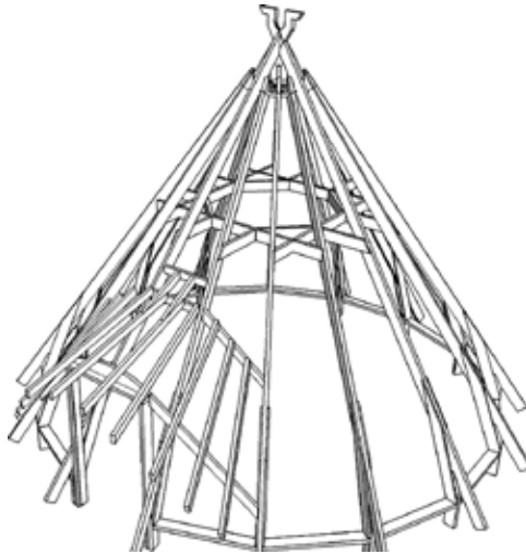
Figure 11. Framework of Svētnīca (under construction) [Žukovskis 2017].
